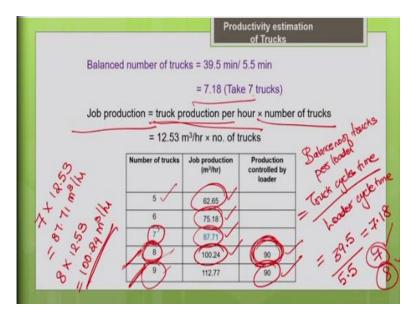
Now let us find the balance number of trucks needed for one loader. So, that depends upon your the balance number of trucks per loader going to be serve by one loader is equal to your truck cycle time divided by load of cycle time. So, you have estimated the truck cycle time earlier, so estimated it is 39.5.
