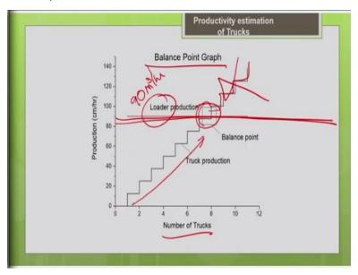
This picture the balance point graph clearly illustrates what is the significance of the balance point. So, as you keep increasing your truck number you can see that the productivity is significantly increasing. At the balance point you can see that the productivity of your truck and the productivity of the loader will be same, loader productivity is 90, the load of productivity is 90-meter cube per hour.
