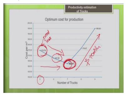
So, graphically you can see this, so when the number of trucks or less your unit protection cost is less when the number of trucks is 5, when the number of trucks is less the unit production cost is higher than the optimum value. You can see the optimum value for the number of trucks 7 the unit production cost is 162.47. But when you go for 5 trucks you can see that the unit production cost is higher than the optimum value, why it is higher than the optimum value?
